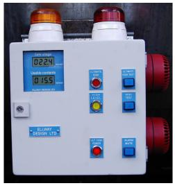
Each level probe and its corresponding alarm are powered from electrically separate sources; typically, the ultimate high level probe is powered from the main plant feed, with the continuous probe taking its feed from the tank heaters. Should one sensor fail the remaining sensor becomes the fail safe\*
