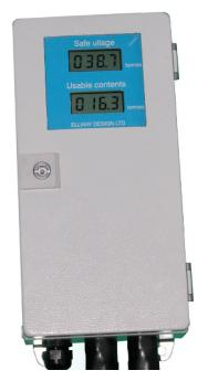
Suitable for use in both vertical and horizontal-cylindrical tanks the microprocessor stores tank shape information and applies the correct linearization calculation to accurately reflect the tank contents.
